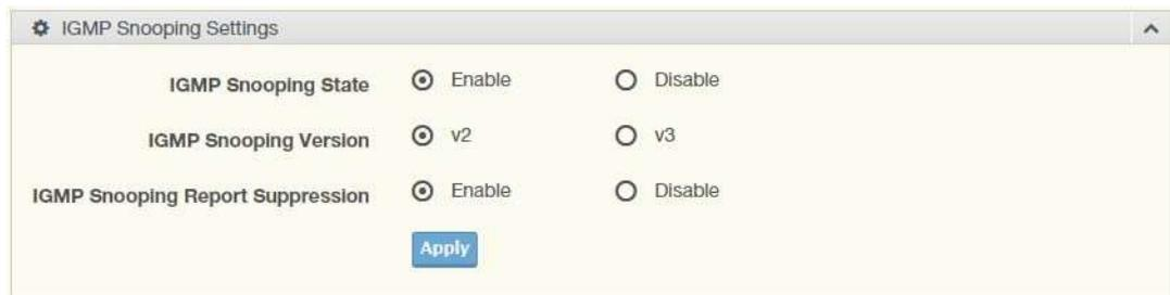
**Figure 3.29 L2 Switching > Multicast > IGMP Snooping > IGMP Settings**
