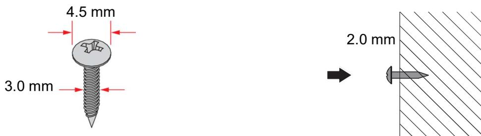
**Figure 2.4 Securing Wall Mounting Screws**
