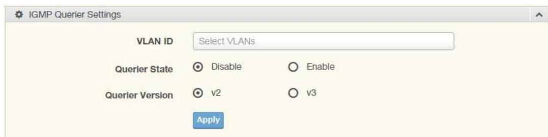
**Figure 3.30 L2 Switching > Multicast > IGMP Snooping > IGMP Querier**
